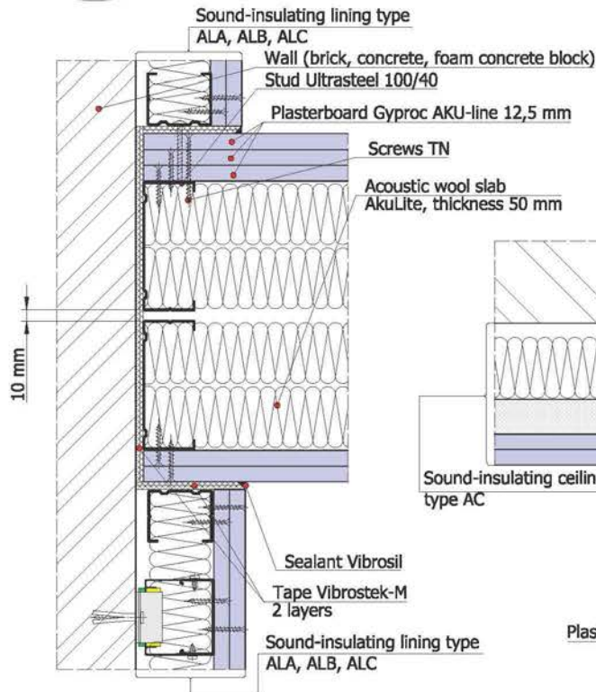
1.20.3 Junction of wall lining to partition
