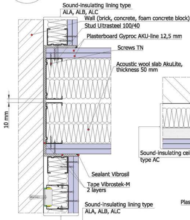
1.19.3 Junction of wall lining to partition
