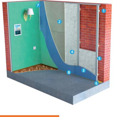
▲R ≈ 24 additional airborne noise insulation airborne noise insulation R<sub>w</sub>≈75 index for the entire construction when mounted on a 120 mm thick sand-lime dB brick wall
