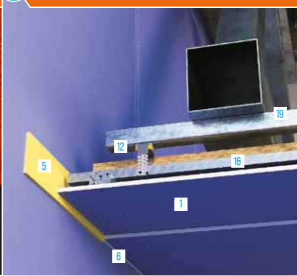
12 FLEXIBLE SOUNDPROOFING CEILING CONNECTION TO THE WALLS
