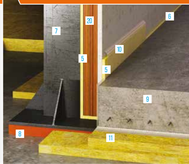
9 FLEXIBLE FLOATING FLOOR CONNECTION TO TIERED SEATING SUPPORTS
