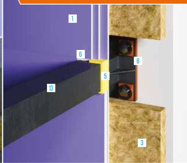
8 VIBRATION ISOLATION OF THE SCREEN FRAME ATTACHMENT TO THE FRONT WALL
